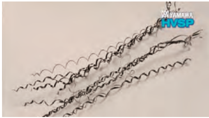
Ejected chips by large size taps
