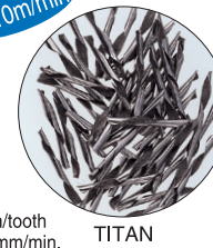
NC5-63 Material: TITAN V=75m/min. f=0.18mm/tooth S=1500min -1 F=1700mm/min.
