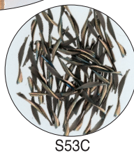
NC5-63 Material: S53C V=500m/min. f=0.25mm/tooth S=10000min -1 F=10000mm/min.
