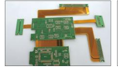
FPC (Flexible printed circuit board)
