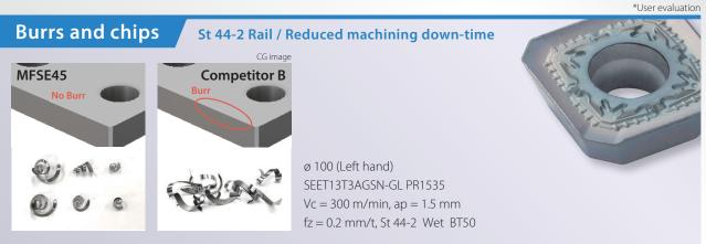
Reduces down-time and reduces burr. Excellent chip control and extended automatic continuous operation time
