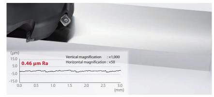
Cutting conditions: Vc = 250 m/min, ap x ae = 1.0 x 100 mm, fz = 0.15 mm/t, wet X5CrNi18-10 ø 125 (Standard 6 inserts) SL Chipbreaker
