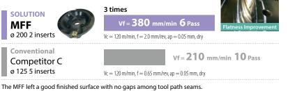
Larger cutter diameter reduced the number of passes to six and improved productivity. Desirable chip shape and size were achieved.
