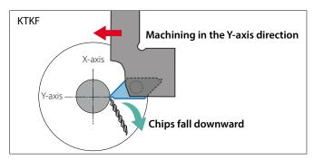
The Y-axis machining direction allows the chips to fall down and away from the workpiece, improving chip evacuation.
