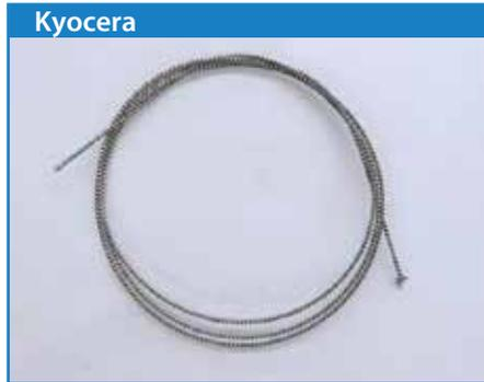
VCGT130302, C45, φ14, Wet, External turning, Vc=140m/min, ap=0.5mm, f=0.07mm/rev, SVJCR1616 type
