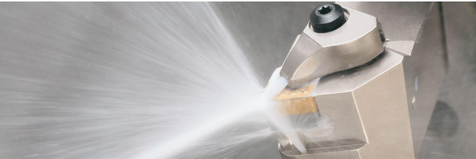
Excellent chip control and long tool life with high pressure coolant
