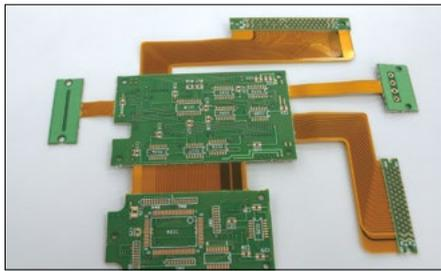
FPC (Flexible printed circuit board)
