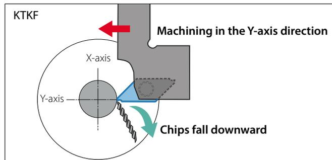
The Y-axis machining direction allows the chips to fall down and away from the workpiece, improving chip evacuation.
