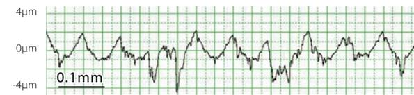
Cutting conditions : Vc = 450 m/min, ap = 0.25 mm, f = 0.10 mm/rev, continuous external turning , wet, workpiece : ADC12 (Die cast aluminum)
