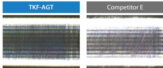
Cutting conditions:  $V_c = 250$  m/min,  $a_p = 2.0$  mm, wet, workpiece: Al-Mg1SiCu
