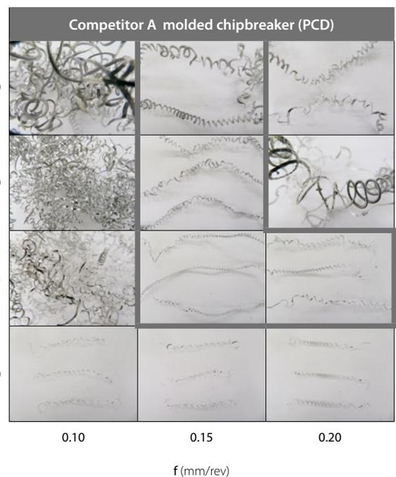
Cutting conditions :  $V_c = 500$  m/min,  $a_p = 0.1 - 1.0$  mm,  $f = 0.10 - 0.20$  mm/rev, continuous external turning , wet, Workpiece: Al-Mg2.5
