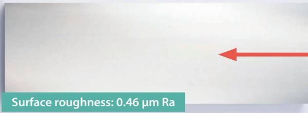
Surface roughness: 0.46  $\mu\text{m Ra}$
