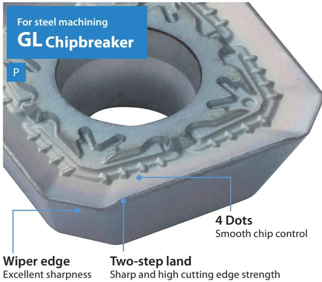
Delivers excellent chip evacuation, sharpness, strength and machining accuracy
