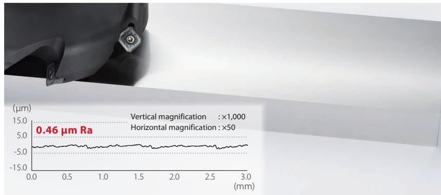
Cutting conditions :  $V_c = 250$  m/min,  $a_p \times a_e = 1.0 \times 100$  mm,  $f_z = 0.15$  mm/t, wet X5CrNi18-10  $\phi 125$  (Standard 6 inserts) SL Chipbreaker
